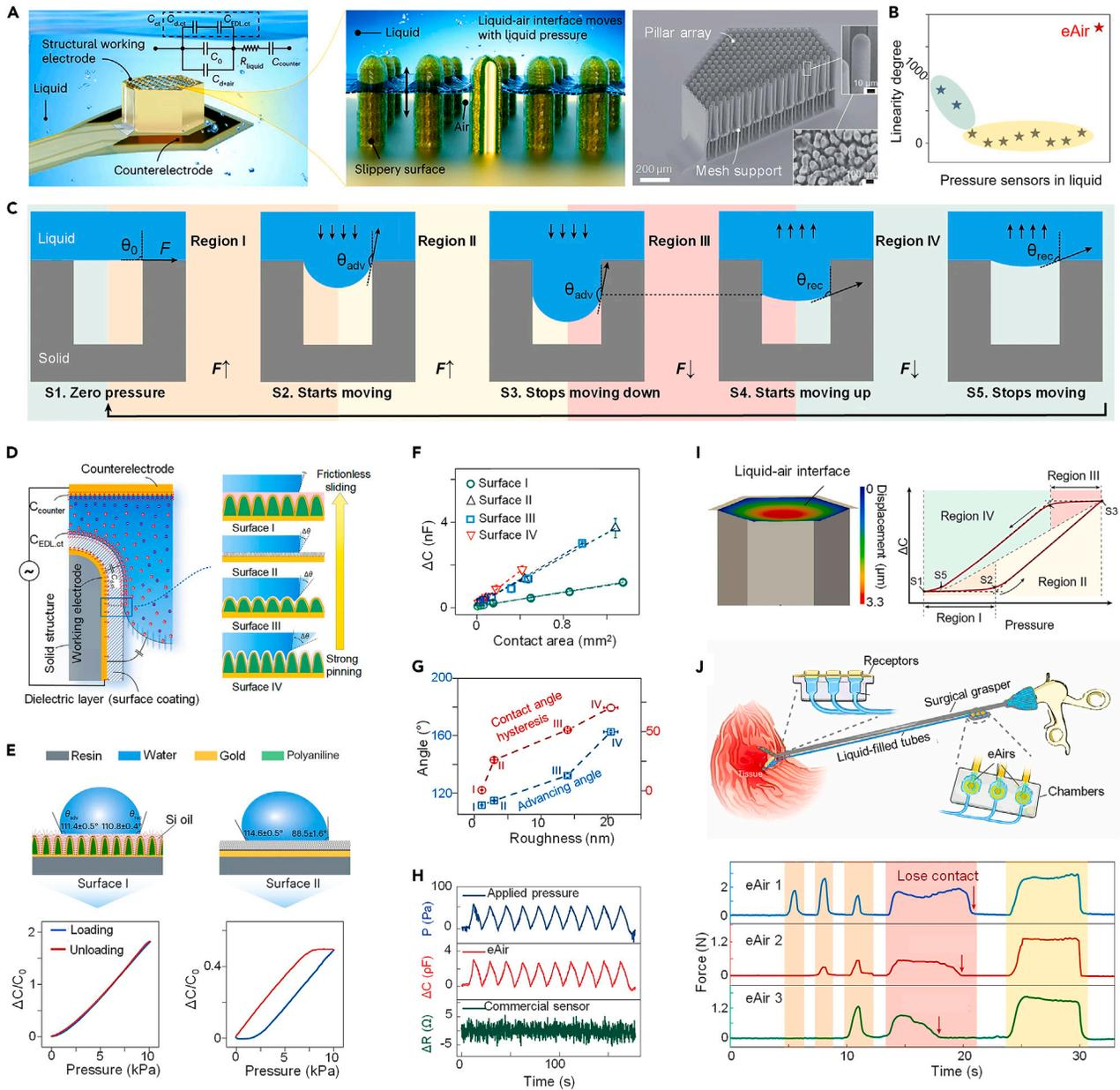
**Figure 1. The aero-elastic capacitive pressure sensor working in aquatic environments**
